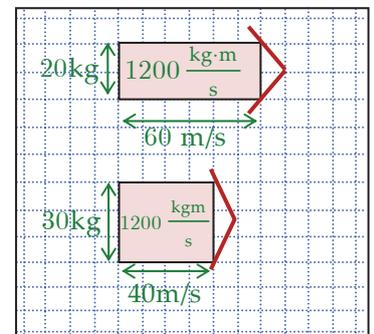
$$p_{in,x} = m_A v_{Ax} = 20 \times 60 \text{ kg m/s} = 1200 \text{ kg m/s}$$
