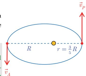
$$\Delta U = \frac{1}{2} m |\vec{v}_A|^2 - \frac{1}{2} m |\vec{v}_P|^2 = \frac{1}{2} m |\vec{v}_P|^2 \left[ 1 - \frac{|\vec{v}_A|^2}{|\vec{v}_P|^2} \right] = \frac{1}{2} m |\vec{v}_P|^2 \left[ 1 - \left( \frac{3}{5} \right)^2 \right] =$$
